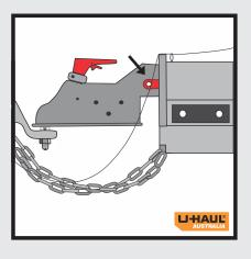
When reversing the trailer/caravan, the latch must be in the CLOSED position to disengage the braking system.
