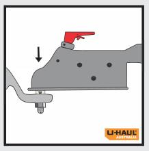
Coupling is now in the locked down position (lock lever horizontal) and ready for towing.
