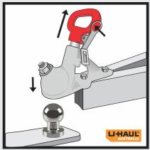
Press coupling handle trigger inwards and pull up handle to enable coupling to be attached or unattached from tow ball.
