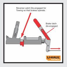
To release handbrake pull handle back and lift ratchet lever (if lever is included) away from locking groves. NB: the ratchet lever must be in this position whilst towing trailer with vehicle.
