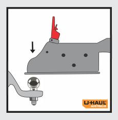
Lift lock lever to unlocked position (vertical) and lower coupling on to a correctly rated 50mm tow ball until locking handle releases to a horizontal position.
