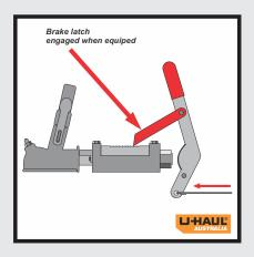
The handbrake is engaged when the handle is pulled back fully and ratchet lever is down in locking groves (if lever is included). NB: wheel chocks MUST always be used also.
