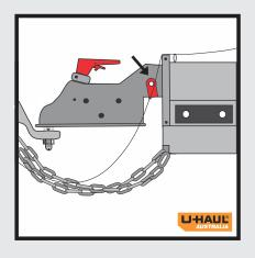
The trailer/caravan brakes are operational when the reverse latch is in the OPEN position.
