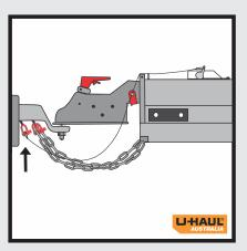
Attach breakaway cable to vehicle separately from the safety chains (do not attach cable to safety chain or D Shackle).
