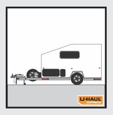
Stabiliser legs raised into travelling position when towing.
