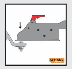
Coupling is now in the locked down position (lock lever horizontal) and ready for towing.
