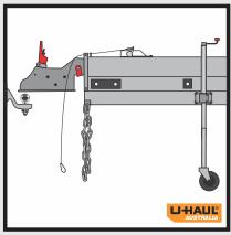
Raise trailer/caravan with jockey wheel /stand to just above tow ball height and reverse vehicle to trailer (do not drag trailer to vehicle). Recommended height of tow ball is between 420mm-460mm).
