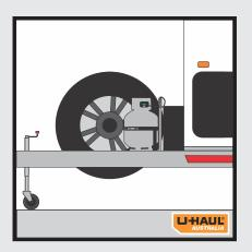
Store hose and electrical cord correctly, and Gas bottle secured and turned off when towing.
