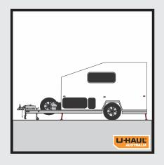
When the caravan is not being towed and in use, it is recommended to use stabiliser legs and wheel chocks to level the caravan.
