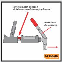
When reversing the trailer, the latch must be in the CLOSED position to disengage the braking system.
