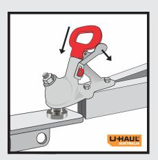
Push handle down and release coupling handle trigger once positioned and lower coupling on to a correctly rated 50mm tow ball. Coupling is now in the locked down position ready for towing.
