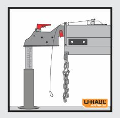
Check caravan tow ball by using the Tow Ball Weight Scale supplied after loading caravan to ensure weight of load is distributed correctly.
